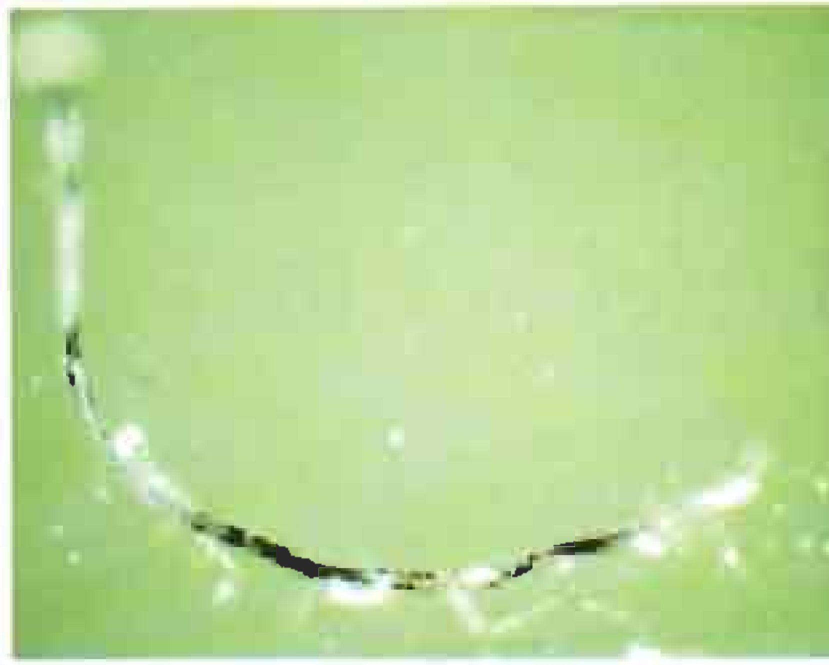
Fig.2 Microscope photograph of a fibre: straw mud, tree cotton, magnification 200x
