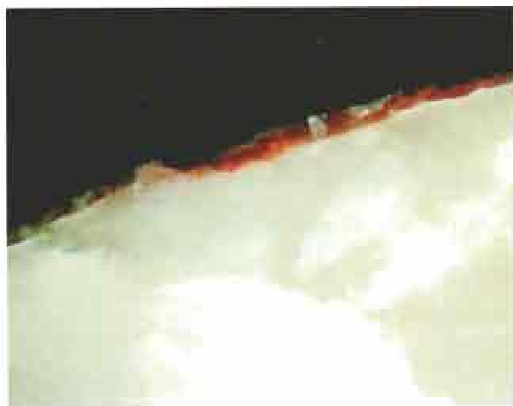
Fig.4 The ground layer of sample YT5 shown fish glue, magnification 500x
