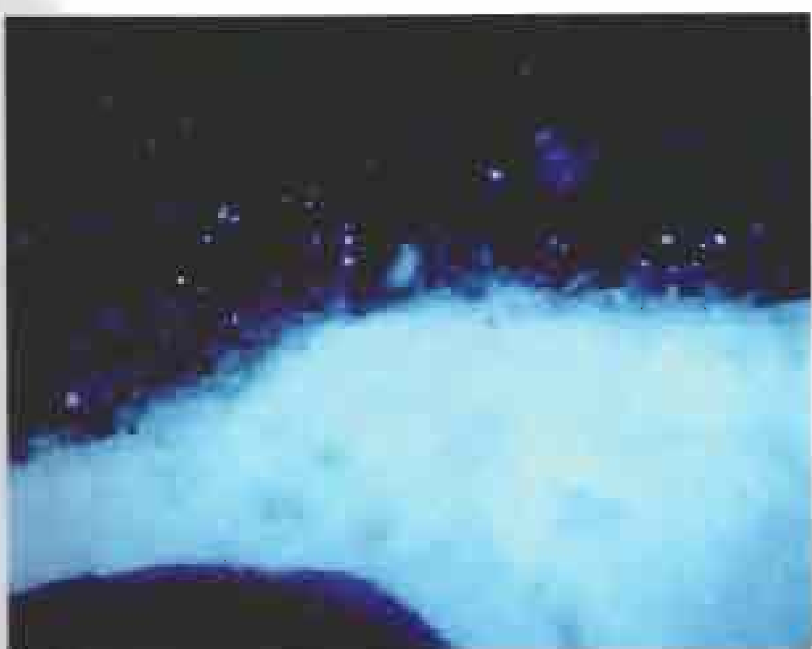
Fig.9 Under UV light the fibres are clearly visible in the layer of losses, yellow earth mixed with three cotton fiber, cotton fibre in this ground layer of the cross section of sample YD3, magnification 200x
