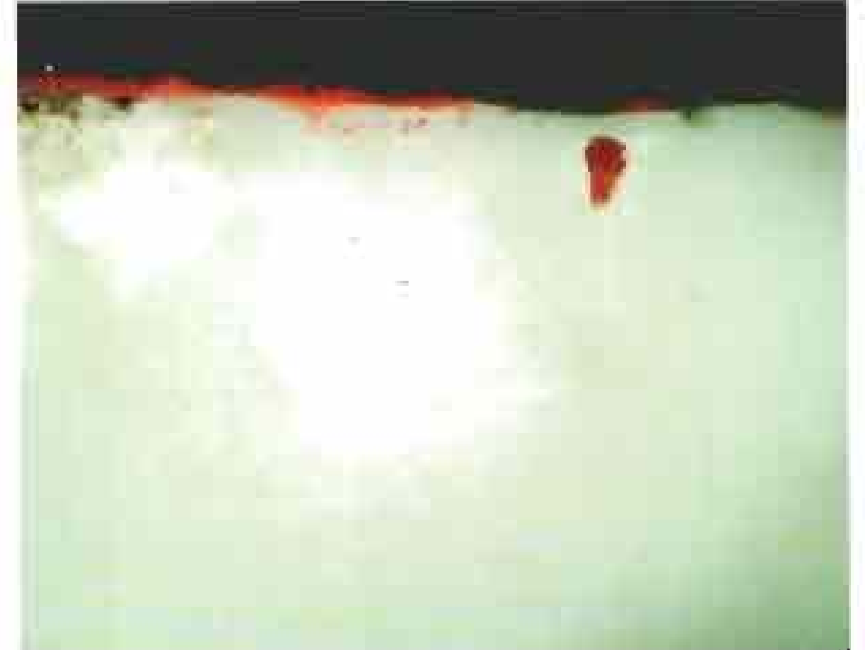
Fig.8 Cross section of sample YD3, showing a remarkable, small spot of lead in the chalk layer. No other traces of lead in any form are present in the samples of the three Tang tombs
